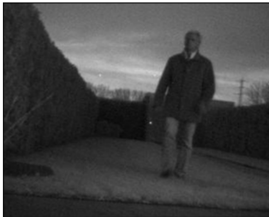
Figure 3: Airglow illumination was enough for this shot on a moonless, starlit night with a sensitive SWIR camera.
