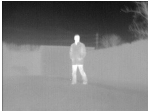
Figure 6: Thermal imaging from an uncooled microbolometer camera can enhance VISWIR images with self-radiating objects.
