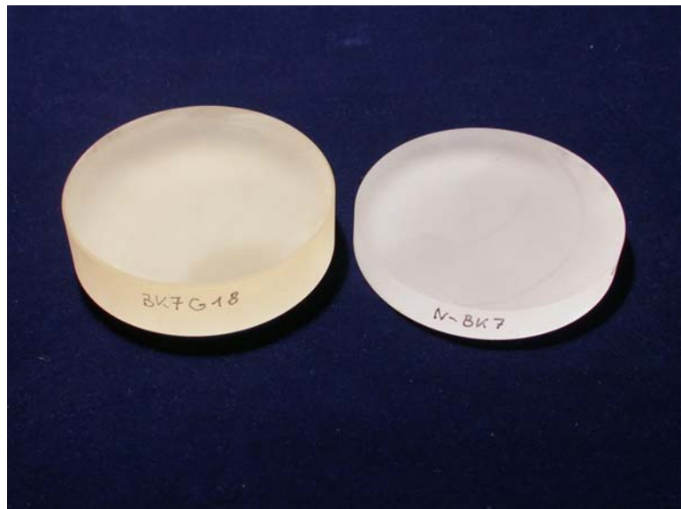
Figure 3-2: Cerium stabilized BK7G18 and non stabilized N-BK7 in direct visual comparison.
