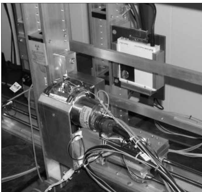
Figure 1 – X-ray system for foam characterization.
