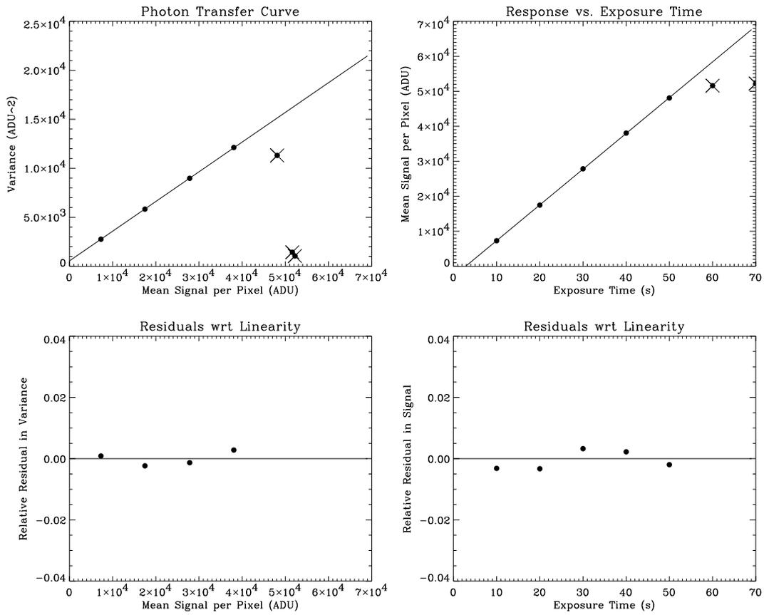
Fig. 4.— Performance curves for the GENII Camera, Amplifier D, Gain Setting 1.0.
