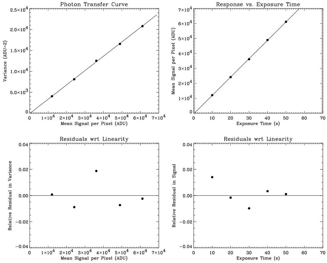
Fig. 3.— Performance curves for the GENII Camera, Amplifier C, Gain Setting 1.0.
