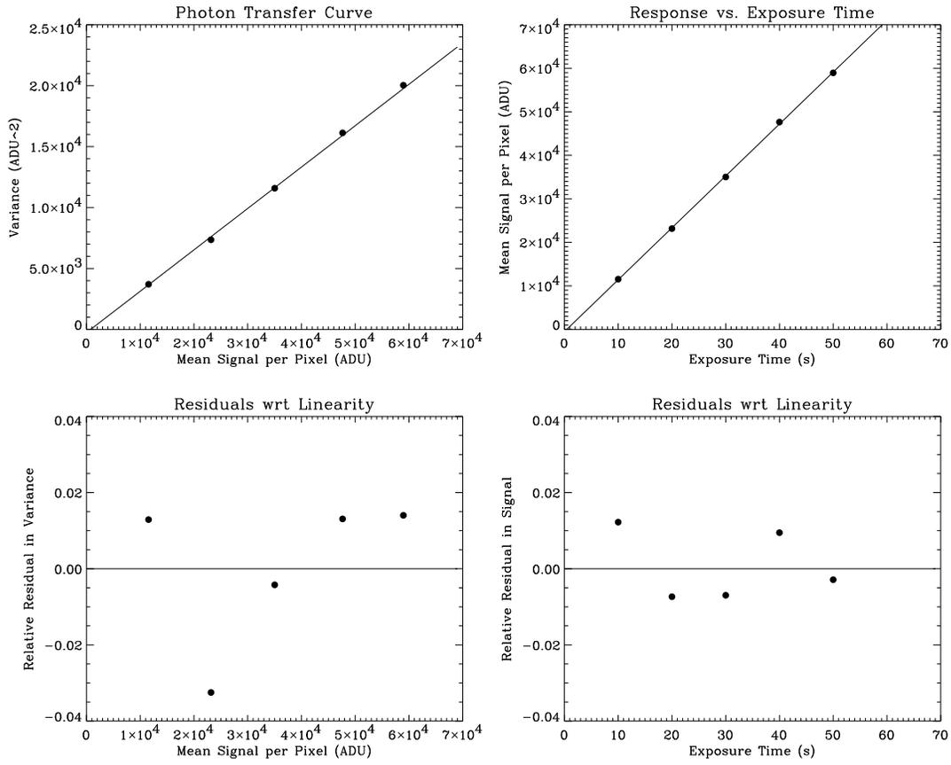
Fig. 1.— Performance curves for the GENII Camera, Amplifier A, Gain Setting 1.0.
