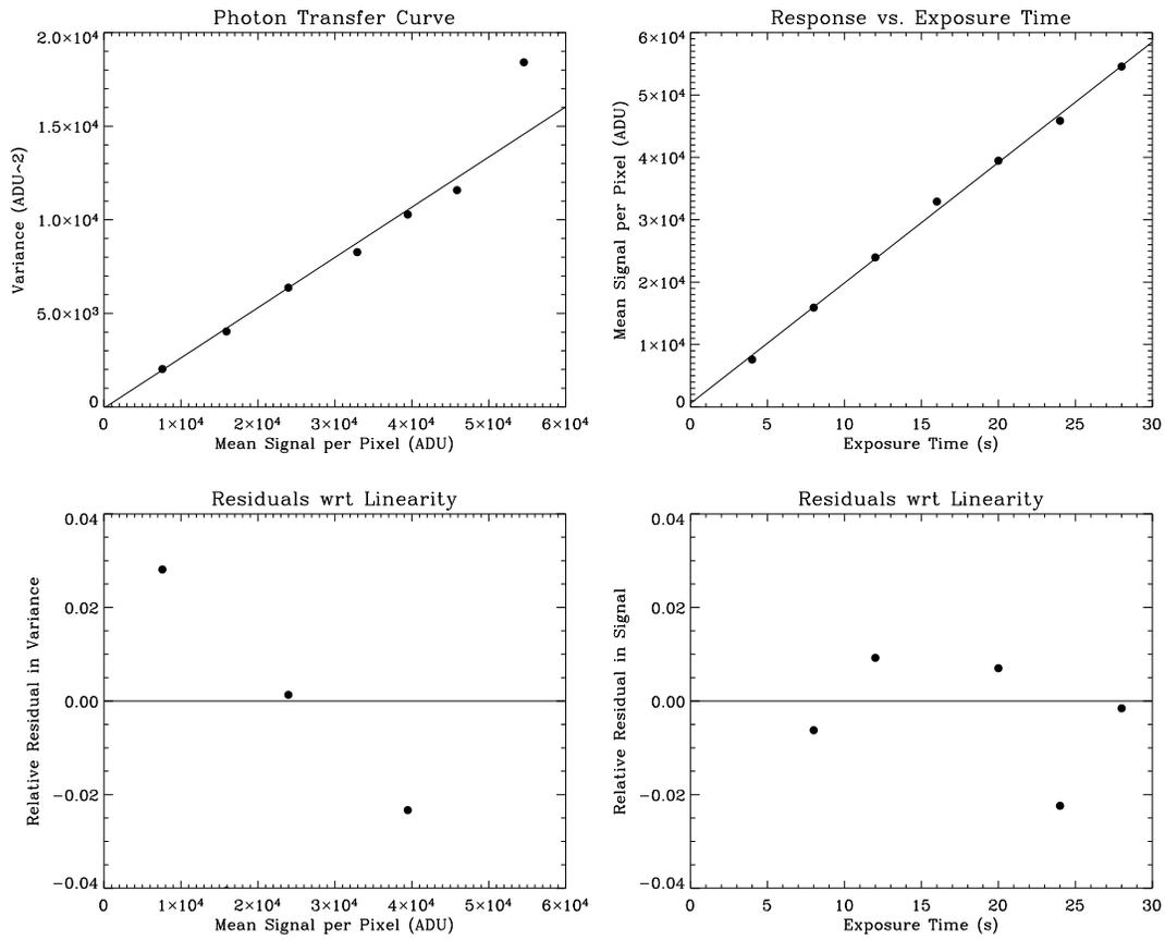
Fig. 5.— Performance curves for the GENI Camera, LOW gain, Trial 1.
