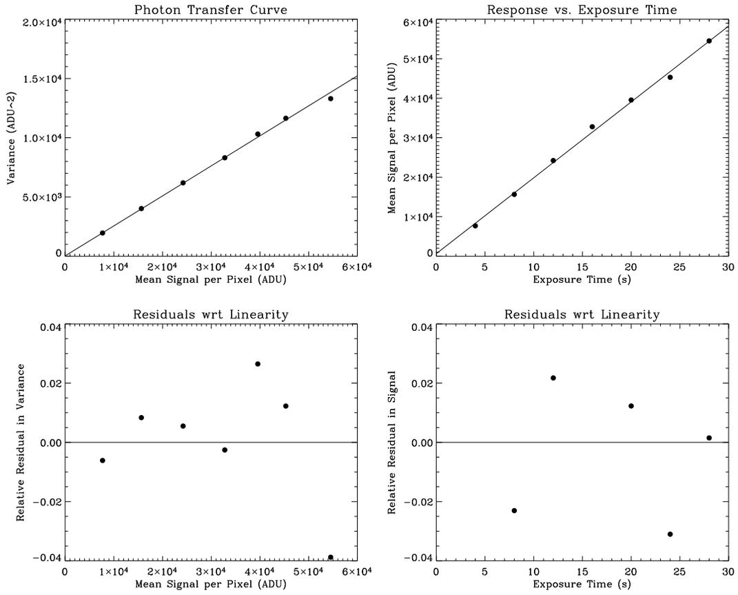
Fig. 6.— Performance curves for the GENI Camera, LOW gain, Trial 2.
