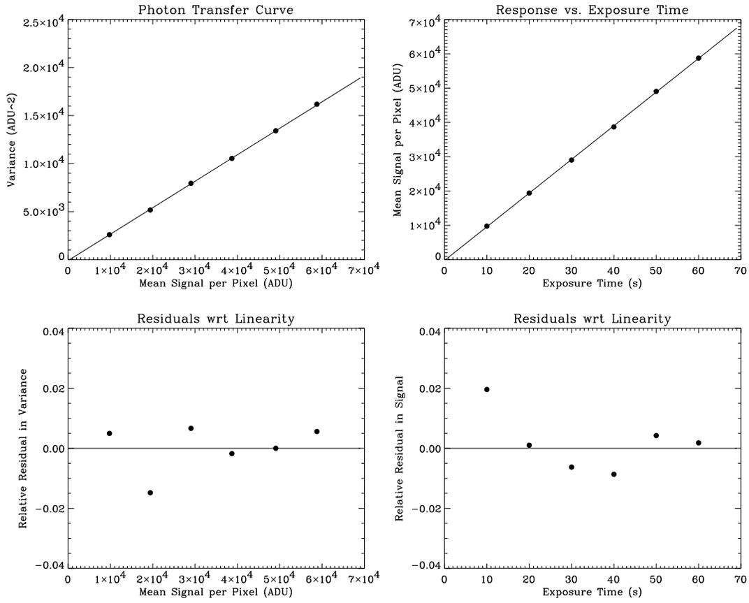
Fig. 2.— Performance curves for the GENII Camera, Amplifier B, Gain Setting 1.0.
