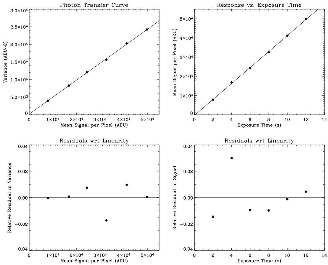
Fig. 9.— Performance curves for the GENI Camera, HIGH gain, Trial 2.
