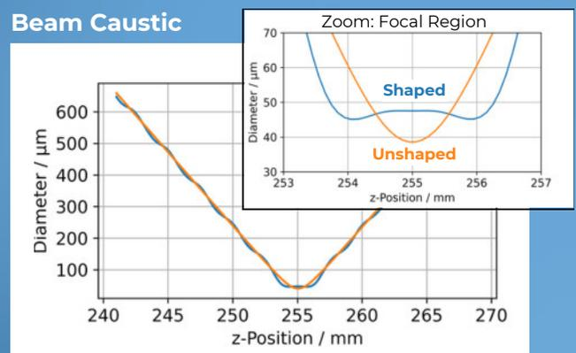
Plotted values for  $\lambda=1070$  nm,  $M2=1.4$ ,  $f=255$  mm, beam diameter=12 mm ( $1/e^2$ )
